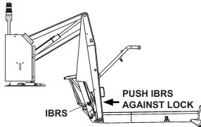
5. On the inboard rollstop switch, loosen screws (1) and (2) one-half turn (FIG. 47-2B). Next, rotate switch bracket clockwise until the switch activates with an audible "click". Then tighten screws (1) and (2) securely.
